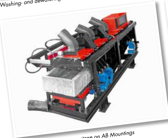
Circular motion screen for gravel on AB TWIN Mountings
