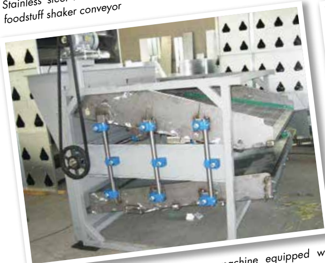
20-meter long two mass shaker conveyor for tobacco leaves equipped with double rocker arms AD-PV 45
