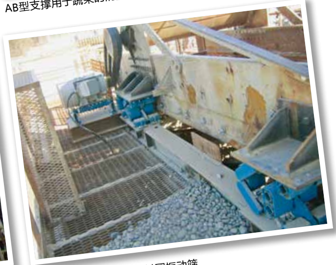
AB TWIN型支撑用于石料圆振动筛
